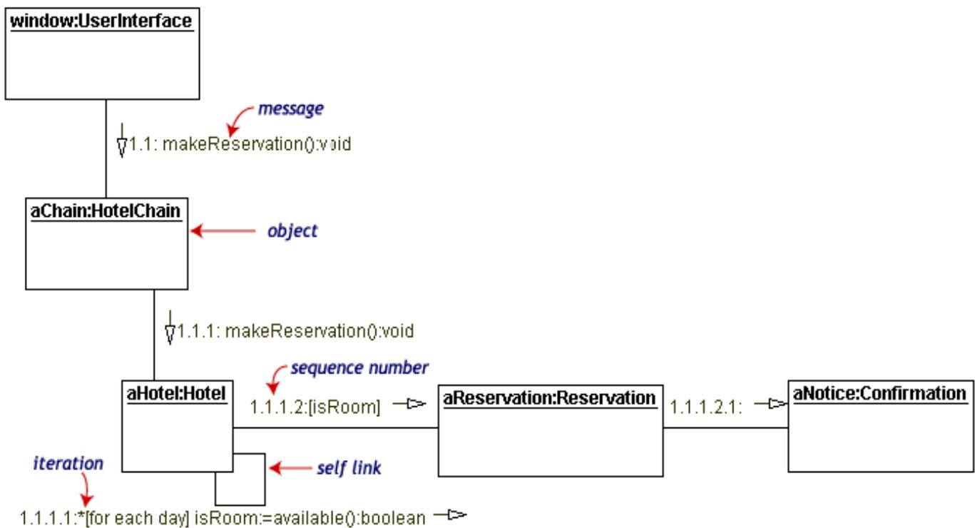
The object-role rectangles are labeled with either class or object names (or both). Class names are preceded by colons ( : ).
