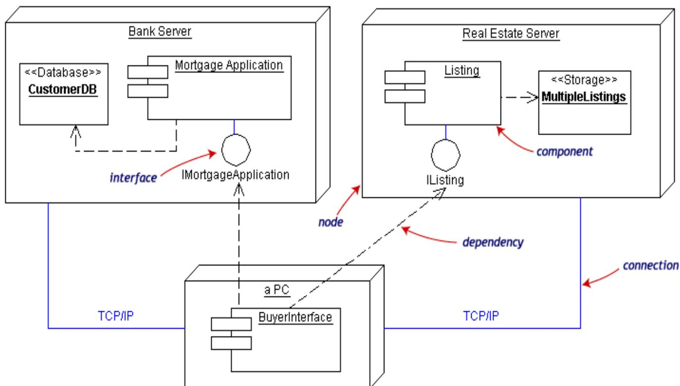
The physical hardware is made up of **nodes**. Each component belongs on a node. Components are shown as rectangles with two tabs at the upper left.
