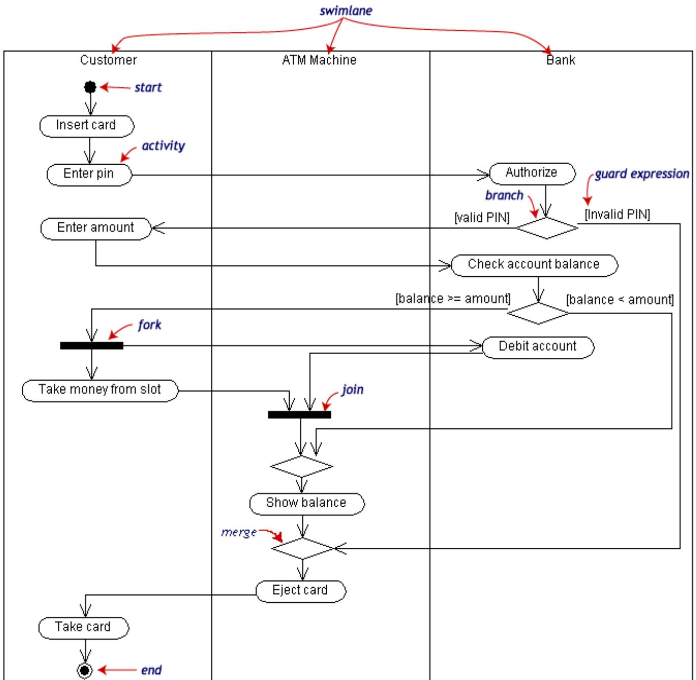
Activity diagrams can be divided into object **swimlanes** that determine which object is responsible for which activity. A single **transition** comes out of each activity, connecting it to the next activity.
