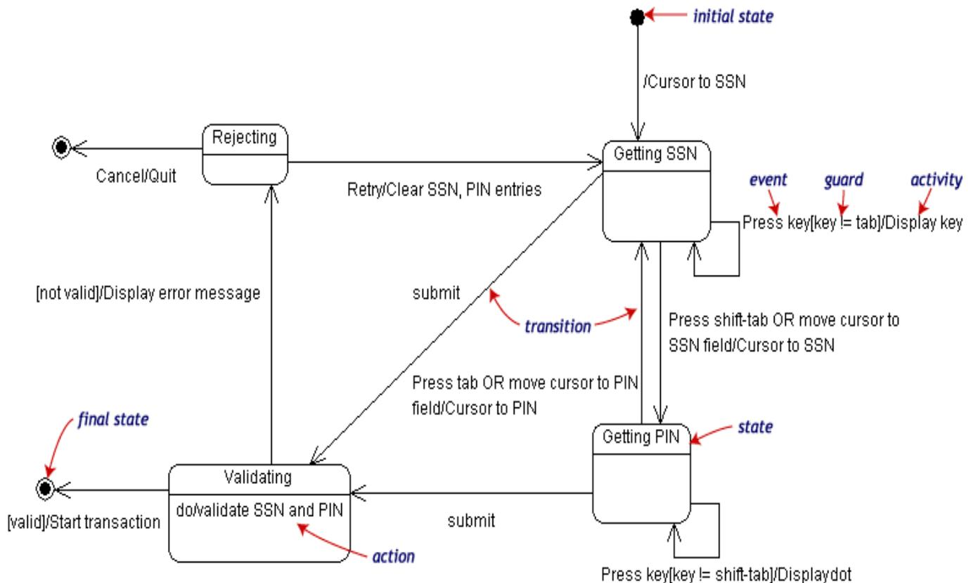
States are rounded rectangles. Transitions are arrows from one state to another. Events or conditions that trigger transitions are written beside the arrows. Our diagram has two self-transition, one on **Getting SSN** and another on **Getting PIN**.
