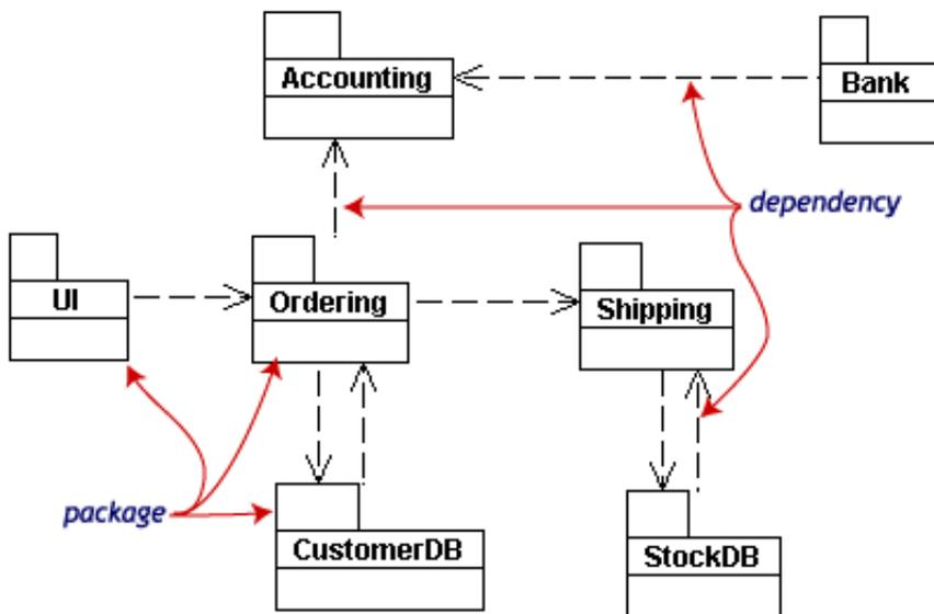
Packages appear as rectangles with small tabs at the top. The package name is on the tab or inside the rectangle. The dotted arrows are **dependencies**. One package depends on another if changes in the other could possibly force changes in the first.
